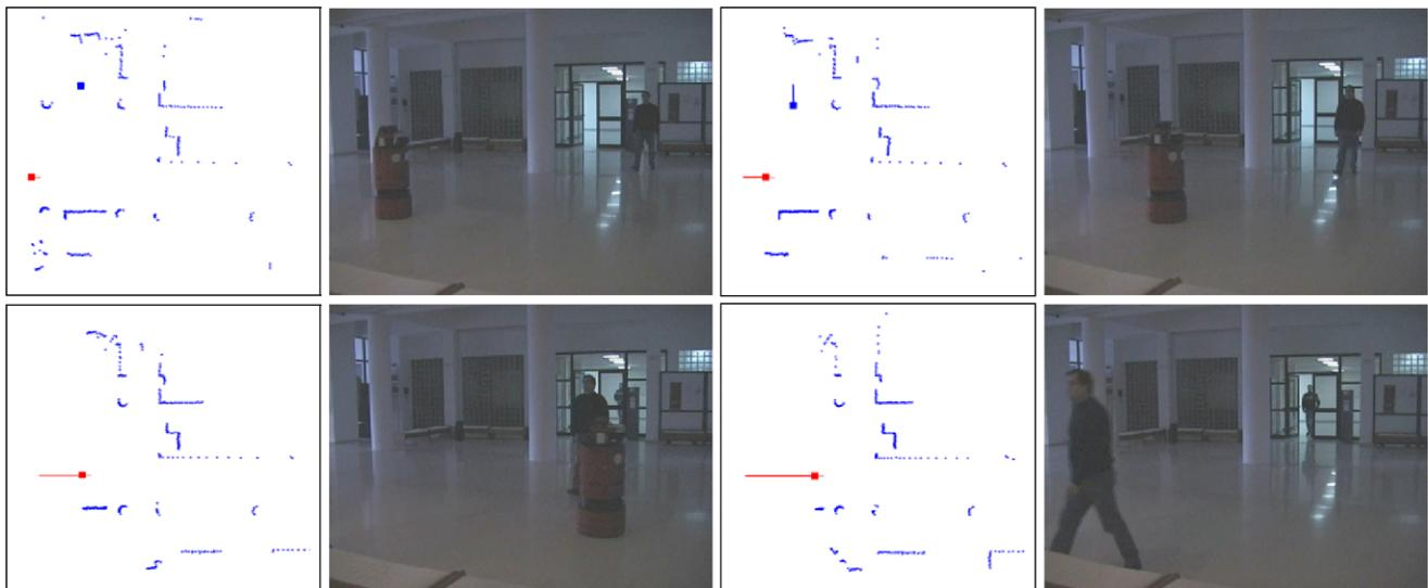
**Fig. 11** Avoiding obstacles by increasing the robot's speed. The robot has to reach the stairs by following a straight path. It detects that a person is coming towards it and decides to increase its speed since it cannot perform a detour or change its path to the goal
