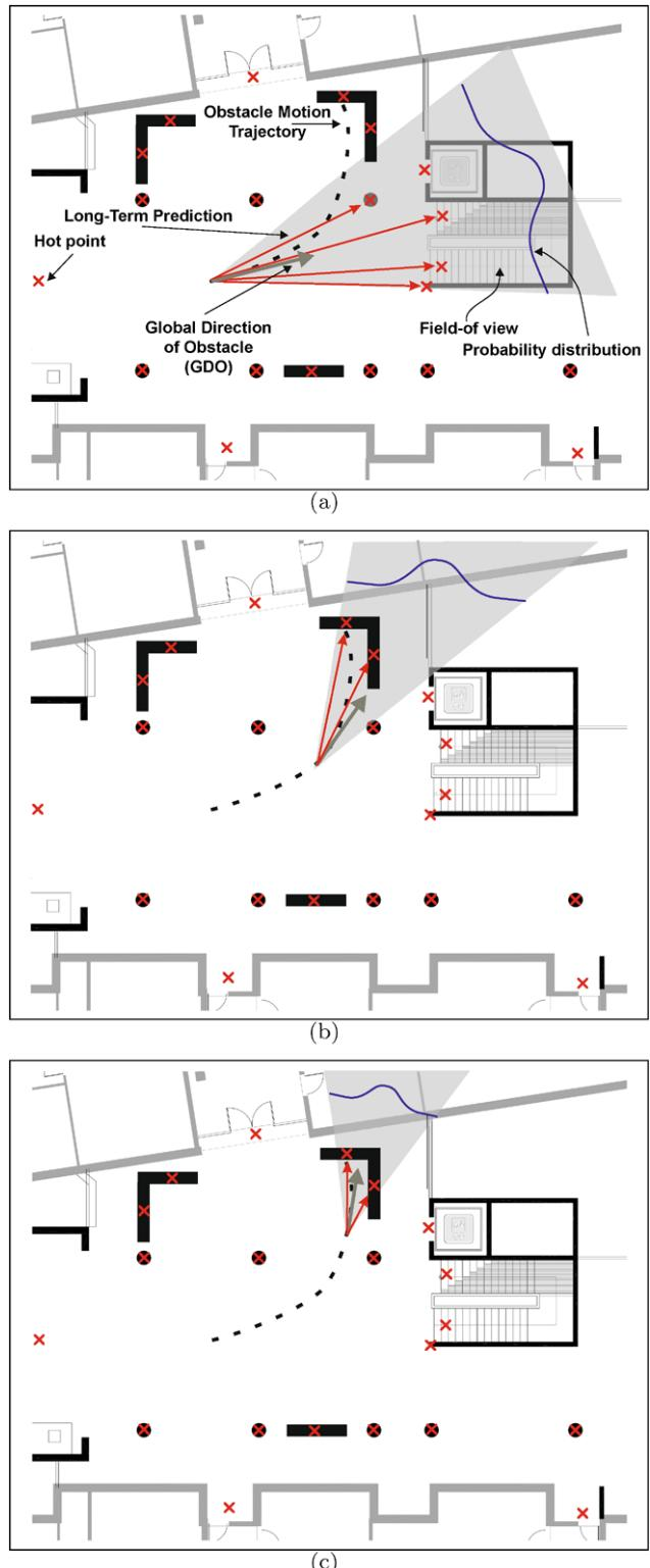
**Fig. 2** An example of making long-term prediction for an object’s movement
