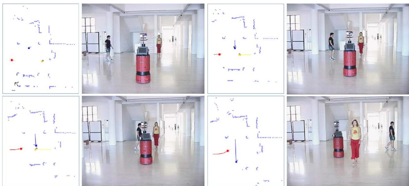
**Fig. 9** Avoiding two moving objects with a detour. The robot detects early in its movement that its path to the goal point, the stairs, will be completely blocked by the two persons moving. Hence, it starts making a detour well before it faces any of the two persons
