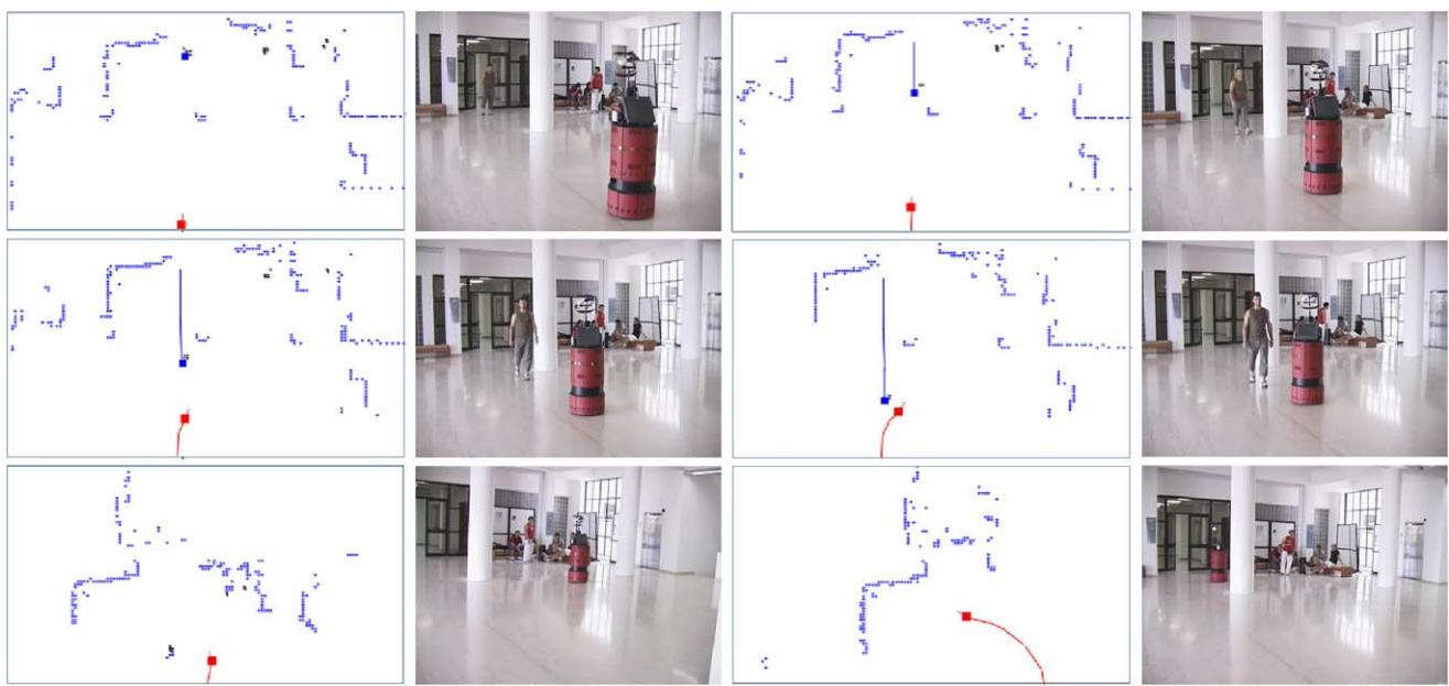
**Fig. 10** Deciding to follow a completely different path. The robot has to follow a simple straight path to reach its goal position that is the starting point of movement of the person present in the environment.
