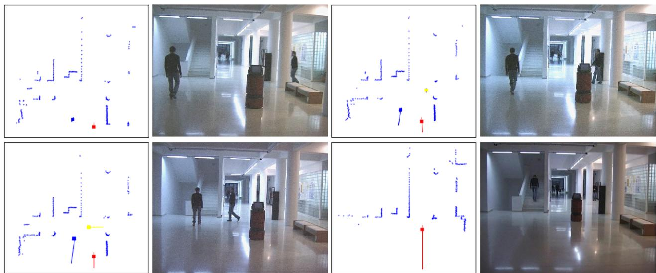
**Fig. 12** Avoiding obstacles by decreasing the robot's speed. The robot has to follow a straight path to reach a distant goal. There is a person moving in parallel with the robot that wants to reach the stairs. Another person's movement that was initially blocked by the building columns
