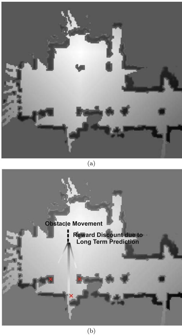
**Fig. 5** (a) The static and (b) dynamic RGM. Reward discount is performed according to the obtained long-term prediction. Long-term predictions for hot points present in the periphery of the field-of-view have low probability,  $w_i$ , and thus the reward discount is smaller
