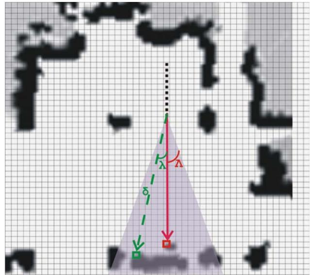
**Fig. 3** The probability assignment for possible hot points is dependent on the angular distance of the considered cell and the GDO and its distance from the obstacle's current position
