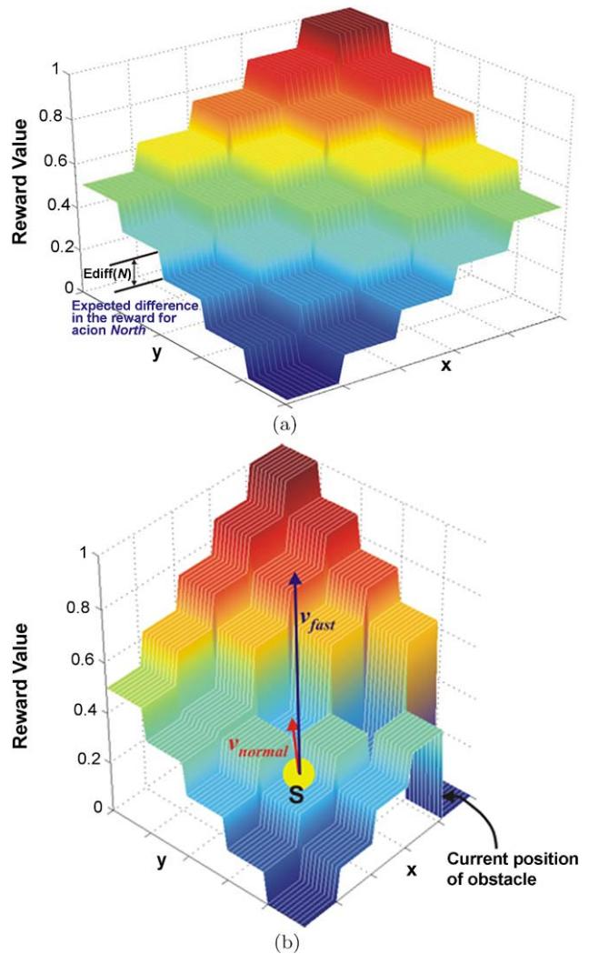
**Fig. 8** (a) The static OGM and (b) an example of the robot choosing to move with the *fast* velocity
